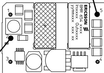
Pin 2 for measurement of maximum peak product reflow temperature,  $T_P$
