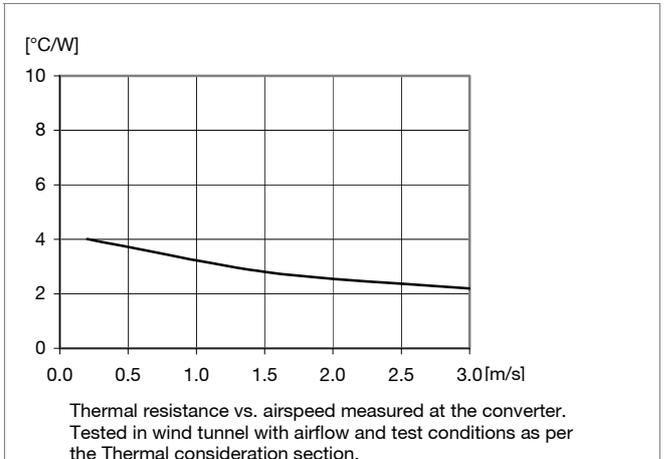
\* Heat sink: finned aluminium, height: 0.23"; Thermal pad: thermal conductivity: 6W/mK, thickness: 0.25mm; Mounting: two M3 screws, torque: 0.44Nm
